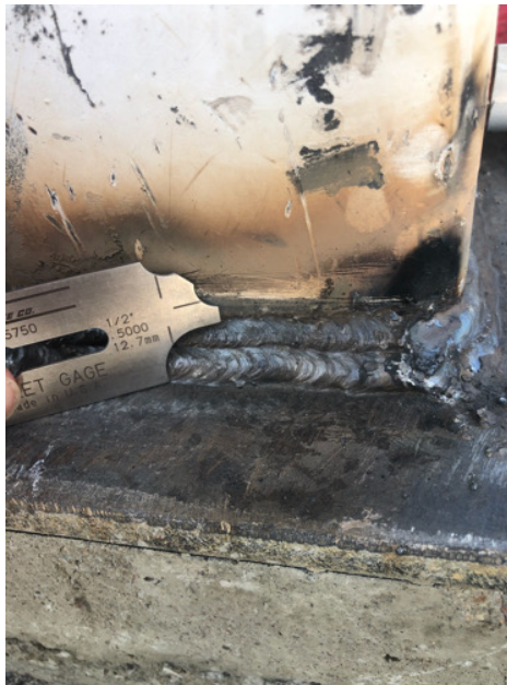
Fig. 8: Column to embed plate fillet weld - guard shack
